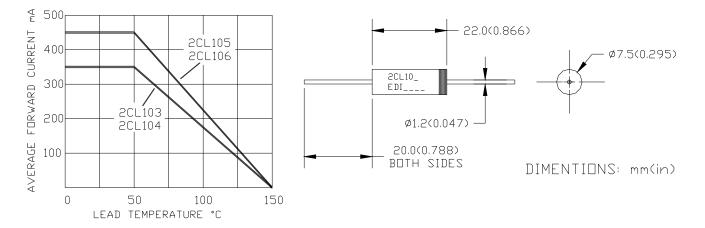
NOTES: It is recommended that a proper heat sink be used on the terminals of this device between the body and the soldering point to prevent damage from excess heat.
